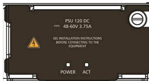
Figure 17 - PSU 120 DC Module
