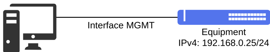
Accessing the equipment using the out-of-band management port
